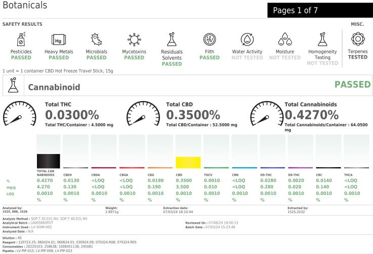
hold analysis utilizing Ultra High Performance Liquid Chromatography with UV Detection (UHPLC-UV). Method SOP.T.30.031.NV for sample preparation and SOP.T.40.031.NV for analysis. Total THC = d8-THC + 0.877 \* THCA, Total CBD = CBD + 0.877 Cannab \* CBDA
